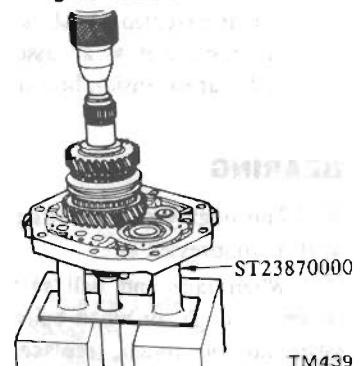
Fig. MT-31 Installing mainshaft assembly
